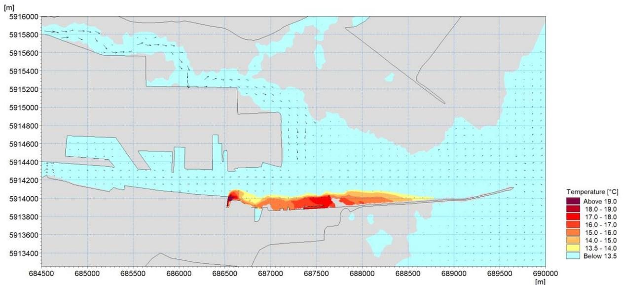
Figure 13.65: Near surface thermal plume envelopes during a typical spring low tide– Post-3FM Project
