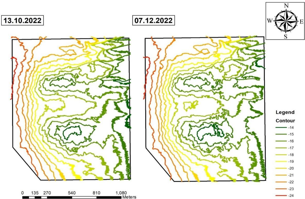
Figure 13.51: Elevation contours of both surveys used to assess the movement of bed material at the dump site
