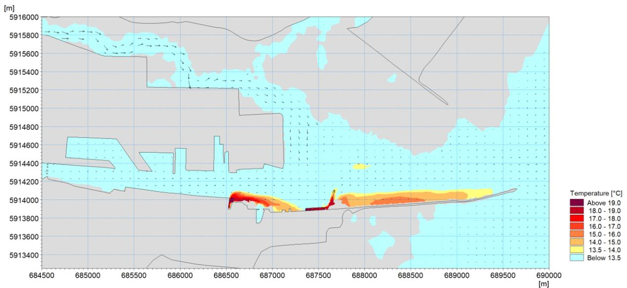
Figure 13.16: Near surface thermal plume envelopes during a typical spring low tide – Pre-3FM Project
