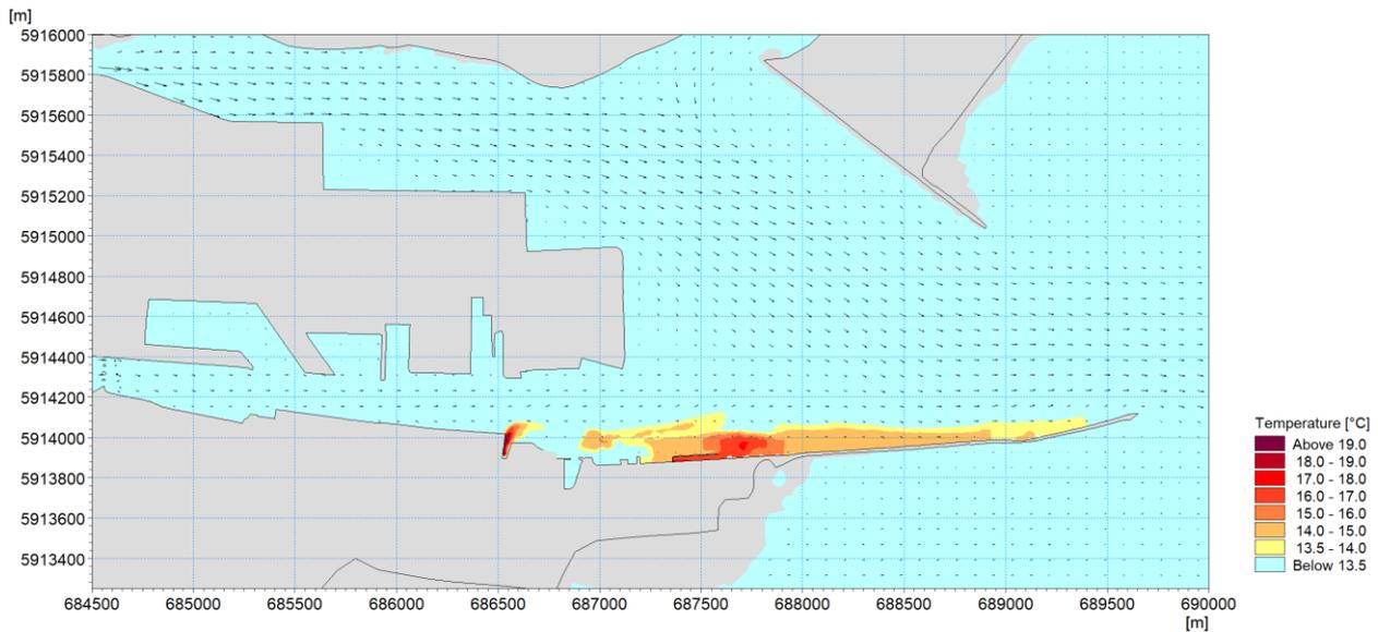
Figure 13.64: Near surface thermal plume envelopes during a typical spring mid ebb tide – Post-3FM Project
