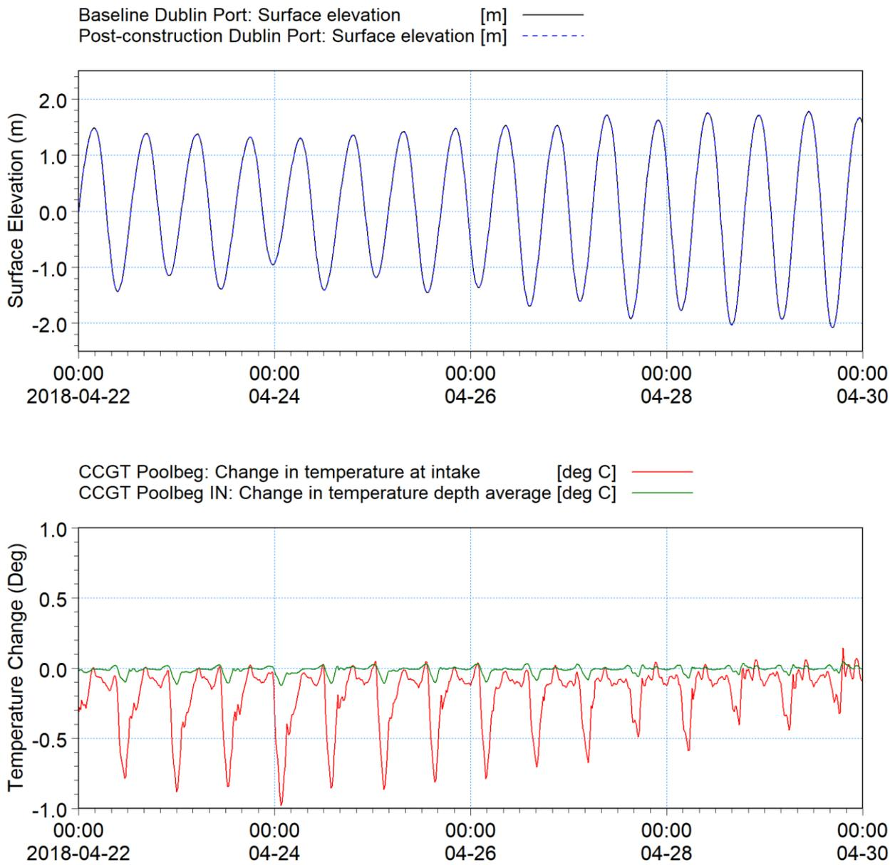
Figure 13.70: Surface elevations (upper) and temperature changes at the Poolbeg intake model layer and average temperature differences across all layers (lower) as a result of the 3FM Project (minus values indicating a temperature decrease relative to baseline conditions and vice versa).
