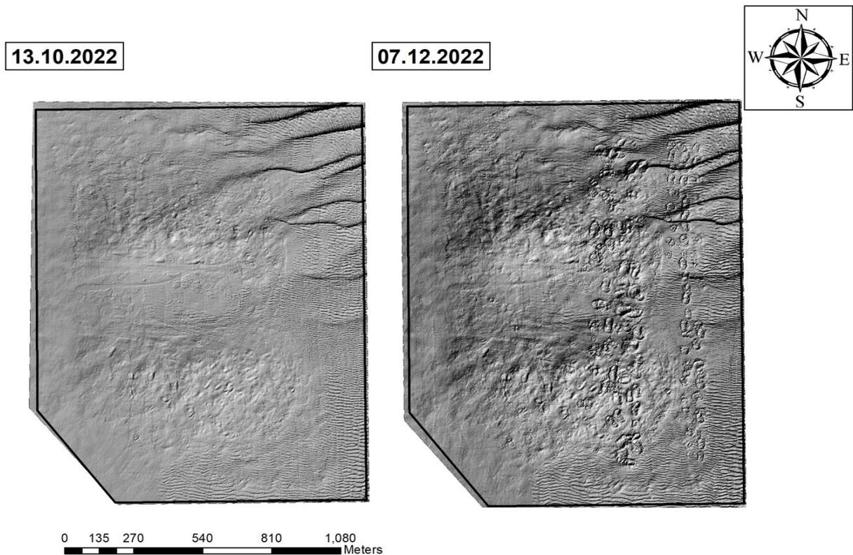
Figure 13.49: Sand wave and other morphological features identified from a terrain analyses of both survey datasets
