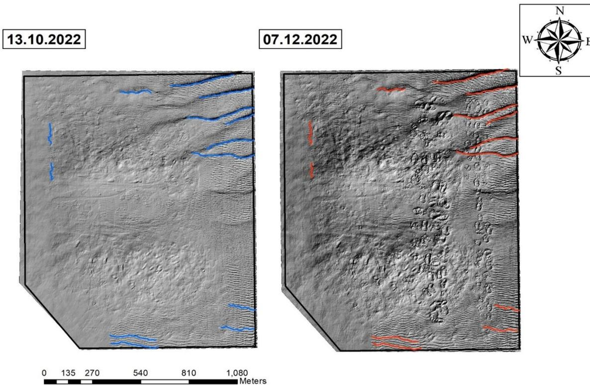
Figure 13.50: Sand wave features common to both surveys identified by blue and red vectors that were used to assess movement of bed material
