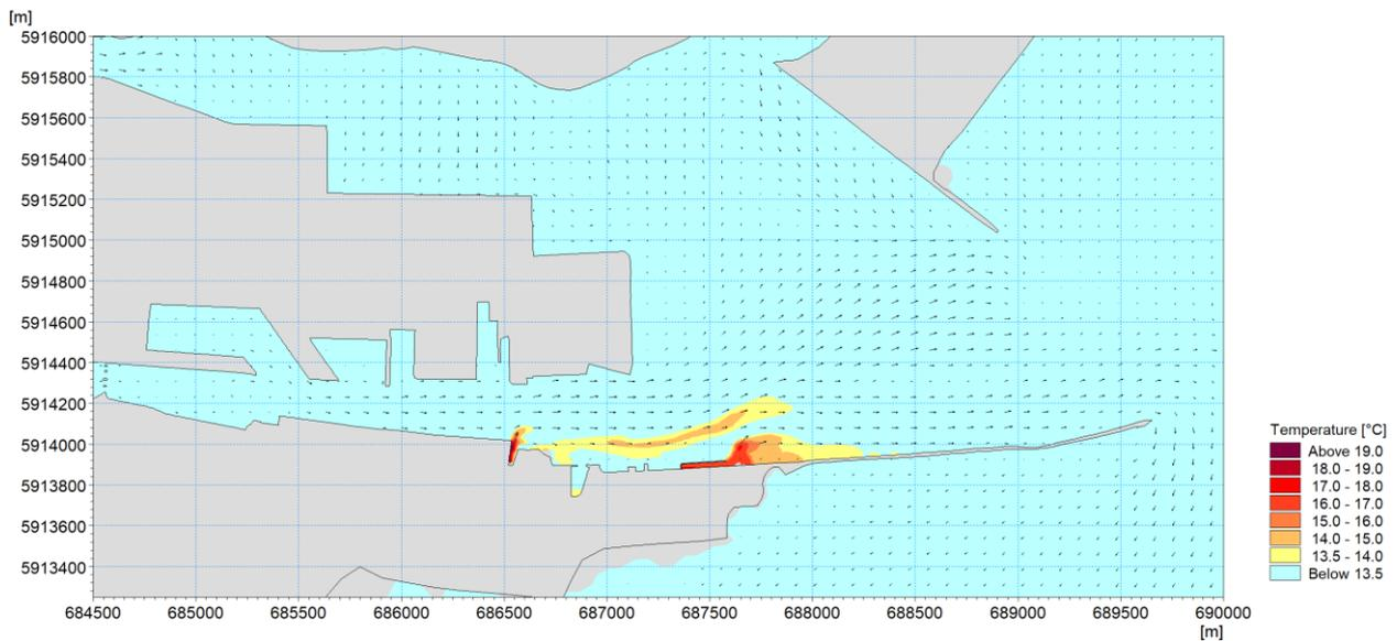
Figure 13.14: Near surface thermal plume envelopes during a typical spring high tide – Pre-3FM Project
